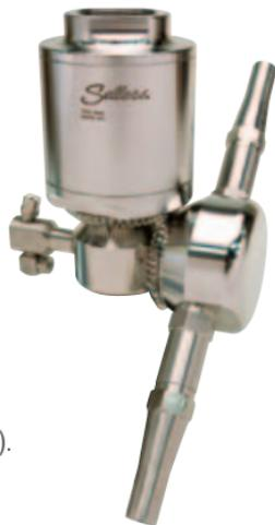
At only 15 lbs (6.8 kgs), the Tankman operates between 60-200 psi (4.1-13.8 bar) and has an effective cleaning diameter of 50 ft (15.2 m).
