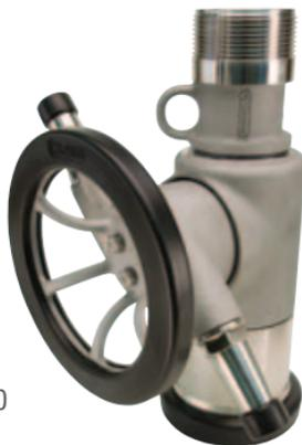
Available with a dual or triple nozzle housing, the Model 700/750 operates with either a self-lubricated flow-through or a sealed oil-lubricated gearbox. Operational ranges include: inlet pressure from 40-500 psi (2.8-34 bar), flows ranging from 40-350 GPM (9-79 m<sup>3</sup>/h) and a cleaning diameter to 100 ft (30 m), at temperature ranges up to 250°F (121°C). Castings are constructed of 316 stainless steel.
