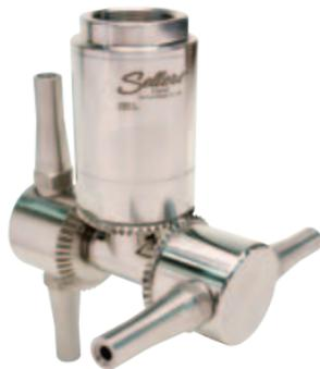
The unit is available in three different nozzle sizes and three different configurations. The recommended operating pressures for the Jumbo 6 is 50-150 psi (3.5-10.3 bar). For applications with extreme temperatures up to 500 degrees, the HT model is the perfect and only choice
